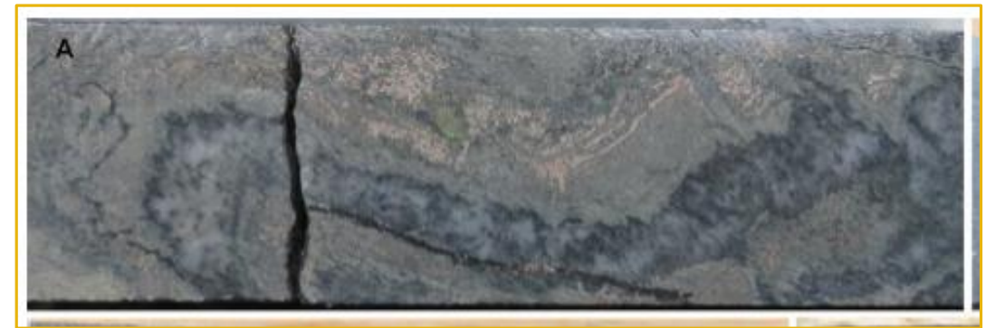
Fine pyrrhotite replacing amphibole altered bands of BIF
